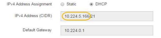
5. Optionally, set a static IP address for the storage controller management port.
