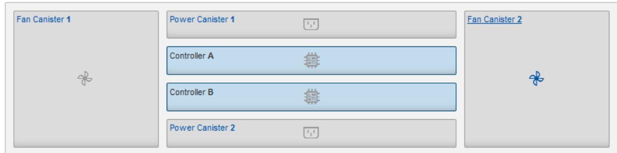
From the back of the shelf, you can view both storage controllers, the battery in each storage controller, the two power canisters, the two fan canisters, and expansion shelves (if any). You can also view component temperatures.
