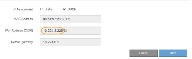
4. Optionally, set a static IP address for the BMC management port.
