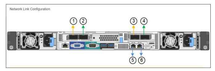
The Link Status table lists the link state and speed of the numbered ports (SG1000 shown).
