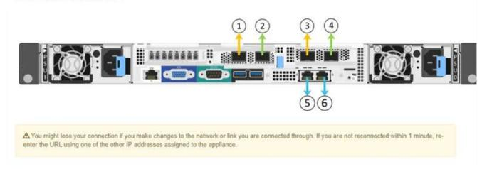
The Link Status table lists the link state (up/down) and speed (1/10/25/40/100 Gbps) of the numbered ports.
