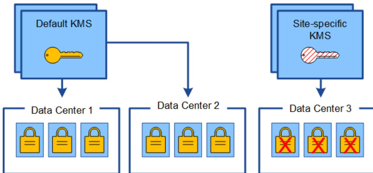
4. To address the issue, you copy the current version of the encryption key from the default KMS to the new KMS. (Technically, you copy the original key to a new key with the same alias. The original key becomes a prior version of the new key.) The site-specific KMS now has the correct key to decrypt the appliance nodes at Data Center 3, so it can be saved in StorageGRID.
