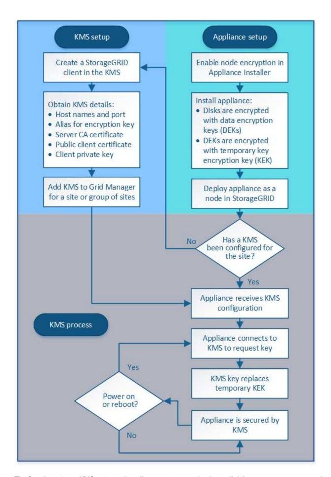
The flowchart shows KMS setup and appliance setup occurring in parallel; however, you can set up the key
