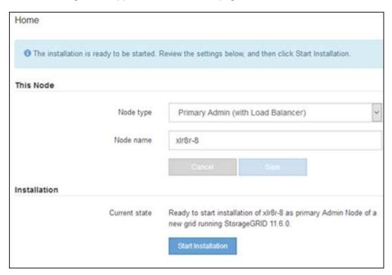
The Current state changes to "Installation is in progress," and the Monitor Installation page is displayed.
