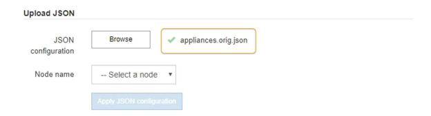
The **Node name** drop down is populated with the top-level node names defined in the JSON file.
