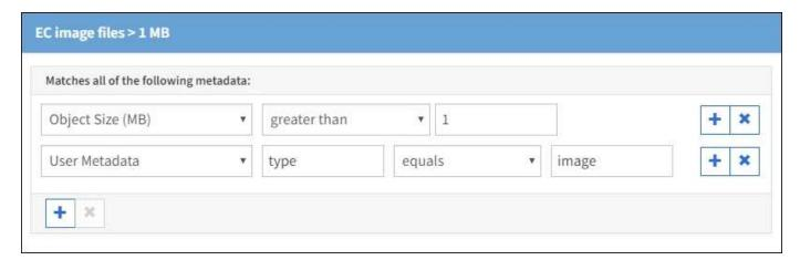
Because this rule is configured as the first rule in the policy, the erasure-coding placement instruction only applies to images that are greater than 1 MB.
