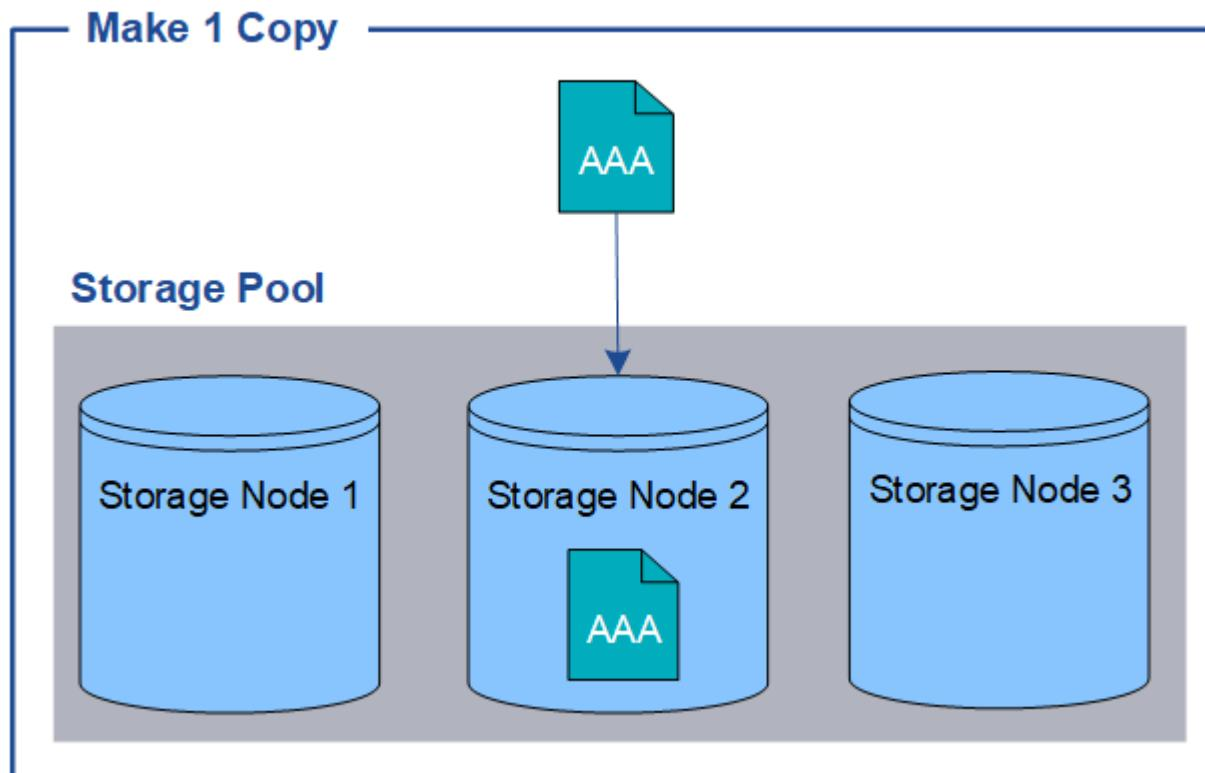
When an ILM rule creates only one replicated copy of an object, the object becomes inaccessible when the Storage Node is unavailable. In this example, you will temporarily lose access to object AAA whenever Storage Node 2 is offline, such as during an upgrade or other maintenance procedure. You will lose object AAA entirely if Storage Node 2 fails.
