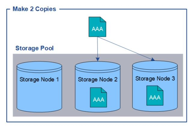
When StorageGRID matches objects to this rule, it creates two copies of the object, placing each copy on a different Storage Node in the storage pool. The two copies might be placed on any two of the three available Storage Nodes. In this case, the rule placed object copies on Storage Nodes 2 and 3. Because there are two copies, the object can be retrieved if any of the nodes in the storage pool fails.
