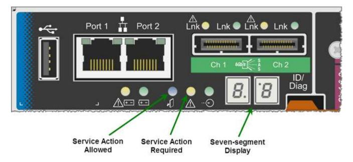
The decimal points on the seven-segment display are not used by the StorageGRID appliance:
