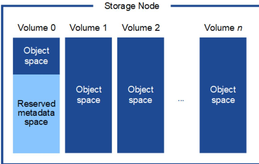
As shown in the figure, StorageGRID reserves space for object metadata on storage volume 0 of each Storage Node. It uses the reserved space to store object metadata and to perform essential database operations. Any remaining space on storage volume 0 and all other storage volumes in the Storage Node are used exclusively for object data (replicated copies and erasure-coded fragments).
