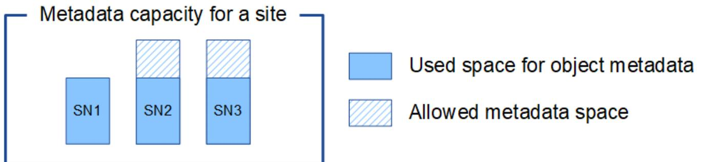
Similarly, because StorageGRID maintains all object metadata for a StorageGRID system at each site, the overall metadata capacity of a StorageGRID system is determined by the object metadata capacity of the smallest site.
