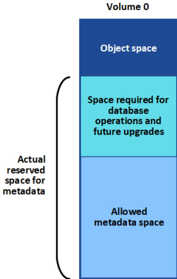
The following table shows how StorageGRID calculates the **allowed metadata space** for different Storage Nodes, based on the amount of memory for the node and the actual reserved space for metadata.
