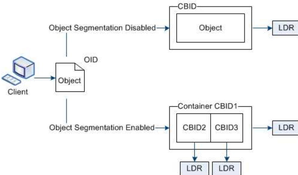
On retrieval of a segment container, the LDR service assembles the original object from its segments and returns the object to the client.
