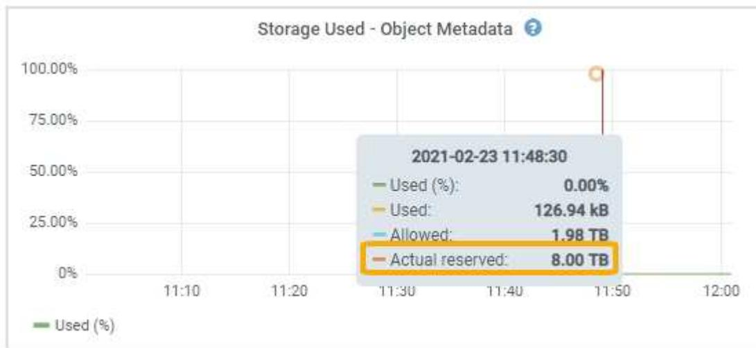
In the screenshot, the **Actual reserved** value is 8 TB. This screenshot is for a large Storage Node in a new StorageGRID 11.6 installation. Because the system-wide Metadata Reserved Space setting is smaller than volume 0 for this Storage Node, the actual reserved space for this node equals the Metadata Reserved Space setting.
