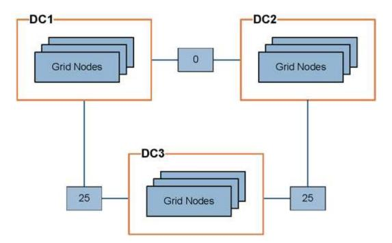
• The CLB service on Gateway Nodes equally distribute client connections to all Storage Nodes at the same data center site and to any data center sites with a link cost of 0.
