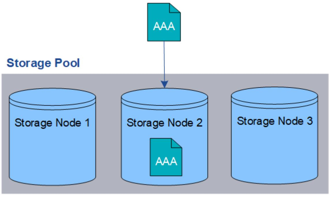
When an ILM rule creates only one replicated copy of an object, the object becomes inaccessible when the Storage Node is unavailable. In this example, you will temporarily lose access to object AAA whenever Storage Node 2 is offline, such as during an upgrade or other maintenance procedure. You will lose object AAA entirely if Storage Node 2 fails.
