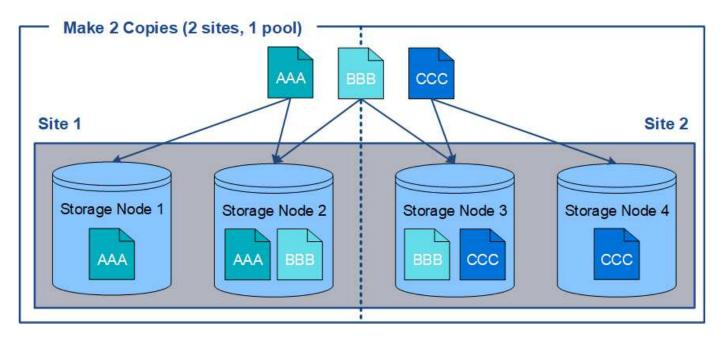
In contrast, this example illustrates how objects are stored when you use multiple storage pools. In the example, the ILM rule specifies that two replicated copies of each object be created, and that the copies be distributed to two storage pools. Each storage pool contains all Storage Nodes at one site. Because a copy of each object is stored at each site, object data is protected from site failure or inaccessibility.
