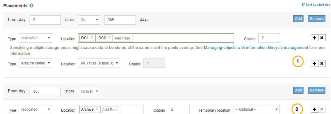
The screenshot shows the 'Placements' section of the Create ILM Rule wizard. It displays two placement rules. Rule 1 (highlighted with a yellow circle) has a 'replicated' type, stores data in 'DC1' and 'DC2' locations, and has 2 copies. Rule 2 (highlighted with a yellow circle) has a 'replicated' type, stores data in an 'Archive' location, and has 2 copies. Both rules have a 'forever' storage duration. The interface includes buttons for 'Add' and 'Remove' placement rules.
