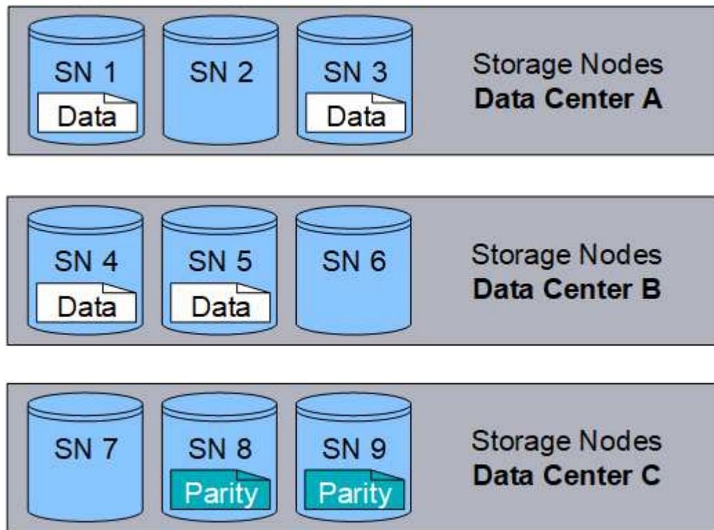
The 4+2 erasure-coding scheme requires a minimum of nine Storage Nodes, with three Storage Nodes at each of three different sites. An object can be retrieved as long as any four of the six fragments (data or parity) remain available. Up to two fragments can be lost without loss of the object data. If an entire data center site is lost, the object can still be retrieved or repaired, as long as all of the other fragments remain accessible.
