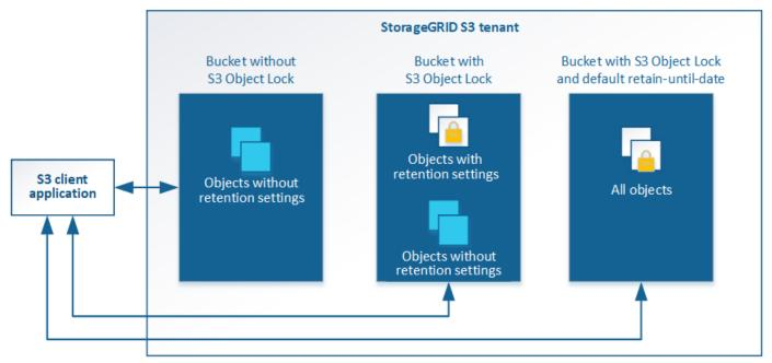
The StorageGRID S3 Object Lock feature provides a single retention mode that is equivalent to the Amazon S3 compliance mode. By default, a protected object version cannot be overwritten or deleted by any user. The StorageGRID S3 Object Lock feature does not support a governance mode, and it does not allow users with special permissions to bypass retention settings or to delete protected objects.
