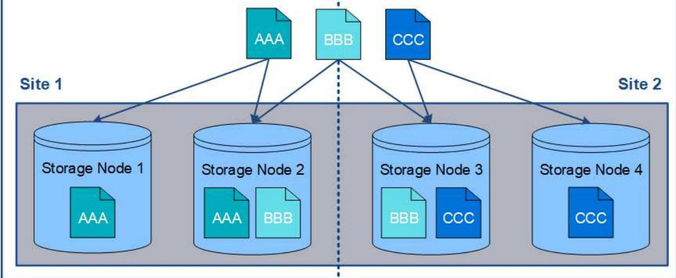
In contrast, this example illustrates how objects are stored when you use multiple storage pools. In the example, the ILM rule specifies that two replicated copies of each object be created, and that the copies be distributed to two storage pools. Each storage pool contains all Storage Nodes at one site. Because a copy of each object is stored at each site, object data is protected from site failure or inaccessibility.
