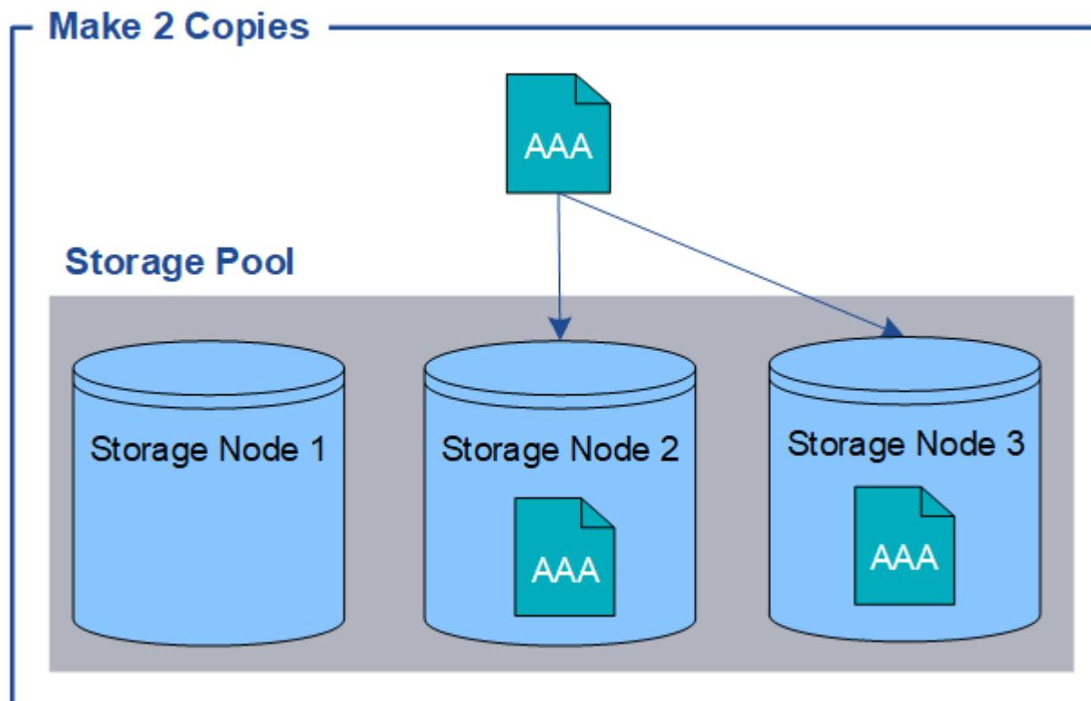
When StorageGRID matches objects to this rule, it creates two copies of the object, placing each copy on a different Storage Node in the storage pool. The two copies might be placed on any two of the three available Storage Nodes. In this case, the rule placed object copies on Storage Nodes 2 and 3. Because there are two copies, the object can be retrieved if any of the nodes in the storage pool fails.
