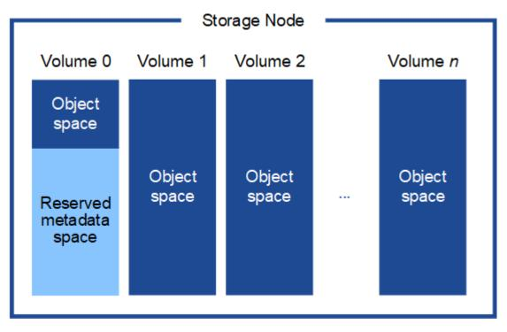
To provide redundancy and to protect object metadata from loss, StorageGRID stores three copies of the metadata for all objects in the system at each site. The three copies of object metadata are evenly distributed across all Storage Nodes at each site.
