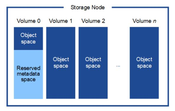
To provide redundancy and to protect object metadata from loss, StorageGRID stores three copies of the metadata for all objects in the system at each site. The three copies of object metadata are evenly distributed across all Storage Nodes at each site.
