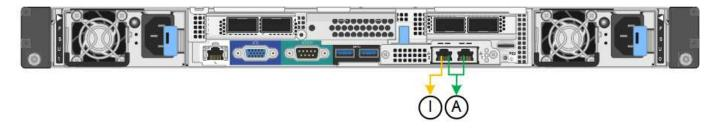
In Independent mode, only the management port on the left is connected to the Admin Network. This mode does not provide a redundant path. The management port on the right is unconnected and available for temporary local connections (uses IP address 169.254.0.1)
