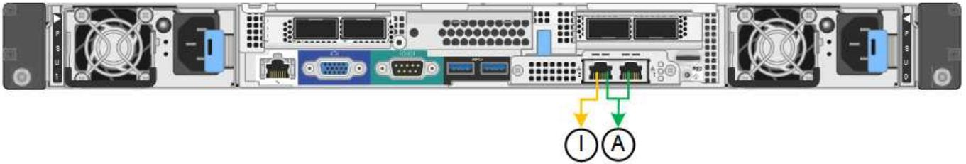
In Independent mode, only the management port on the left is connected to the Admin Network. This mode does not provide a redundant path. The management port on the right is unconnected and available for temporary local connections (uses IP address 169.254.0.1)
