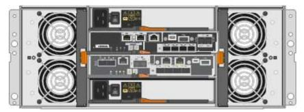
The SG5760S includes two controllers, two fan canisters, and two power canisters.
