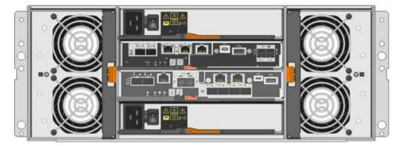
The SG5760 includes two controllers, two fan canisters, and two power canisters.
