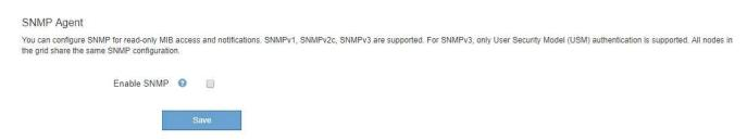
2. To enable the SNMP agent on all grid nodes, select the **Enable SNMP** check box.
