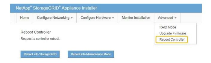
It can take up to 20 minutes for the appliance to reboot and rejoin the grid. To confirm that the reboot is complete and that the node has rejoined the grid, go back to the Grid Manager. The **NODES** page should display a normal status (green check mark icon to the left of the node name) for the appliance node, indicating that no alerts are active and the node is connected to the grid.
