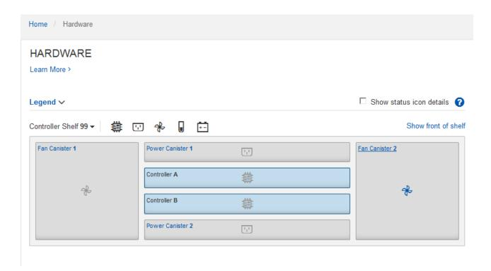
From the back of the shelf, you can view both storage controllers, the battery in each storage controller, the two power canisters, the two fan canisters, and expansion shelves (if any). You can also view component temperatures.
