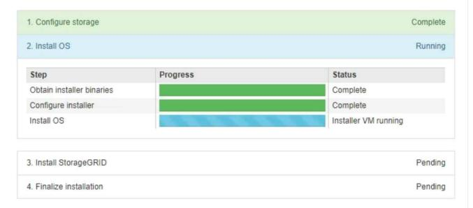
The blue status bar indicates which task is currently in progress. Green status bars indicate tasks that have completed successfully.
