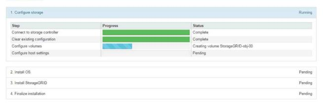
The blue status bar indicates which task is currently in progress. Green status bars indicate tasks that have completed successfully.
