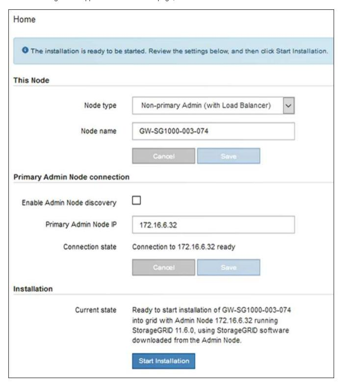
The Current state changes to "Installation is in progress," and the Monitor Installation page is displayed.
