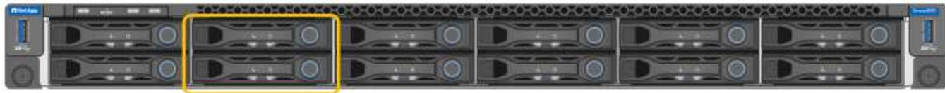
The two solid-state drives (SSDs), indicated by the orange outline, are used for storing the StorageGRID operating system and are mirrored using RAID 1 for redundancy. When the SG100 or SG1000 services appliance is configured as an Admin Node, these drives are used to store audit logs, metrics, and database tables.
