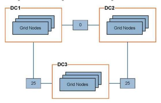
• The Load Balancer service on Admin Nodes and Gateway Nodes equally distributes client connections to all Storage Nodes at the same data center site and to any data center sites with a link cost of 0.
