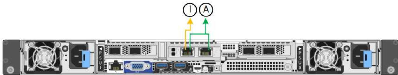
In Independent mode, only the management port on the left is connected to the Admin Network. This mode does not provide a redundant path. The management port on the right is unconnected and available for temporary local connections (uses IP address 169.254.0.1).
