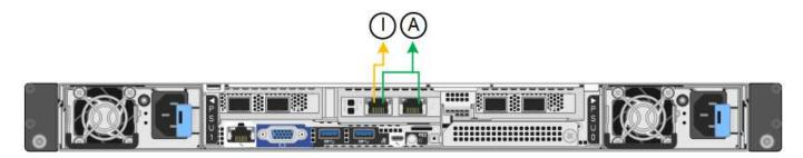
In Independent mode, only the management port on the left is connected to the Admin Network. This mode does not provide a redundant path. The management port on the right is unconnected and available for temporary local connections (uses IP address 169.254.0.1).
