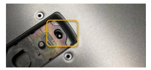
2. Rotate the cover latch forward and down until it stops and the cover fully seats into the chassis. Verify that there are no gaps along the front edge of the cover.
