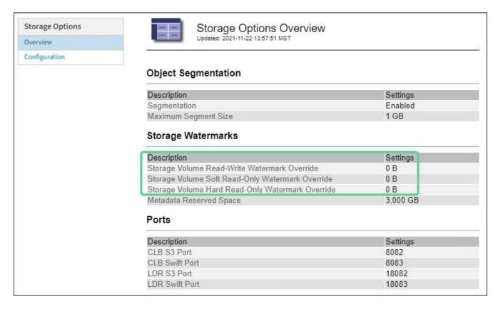
If the watermark overrides are 0, all three watermarks are optimized for every storage volume on every Storage Node, based on the size of the Storage Node and the relative capacity of the volume.
