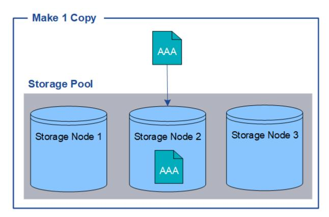
When an ILM rule creates only one replicated copy of an object, the object becomes inaccessible when the Storage Node is unavailable. In this example, you will temporarily lose access to object AAA whenever Storage Node 2 is offline, such as during an upgrade or other maintenance procedure. You will lose object AAA entirely if Storage Node 2 fails.
