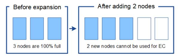
To make use of the new Storage Nodes, you should run the EC rebalance procedure. When this procedure runs, StorageGRID redistributes existing erasure-coded data and parity fragments among all Storage Nodes at the site. In this example, when the EC rebalance procedure is complete, all five nodes are now only 60% full,
