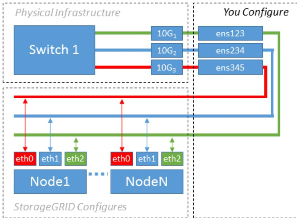
The Linux operating system creates the `ensXYZ` interfaces automatically during installation or boot, or when the interfaces are hot-added. No configuration is required other than ensuring that the interfaces are set to come up automatically after boot. You do have to determine which `ensXYZ` corresponds to which StorageGRID network (Grid, Admin, or Client) so you can provide the correct mappings later in the configuration process.
