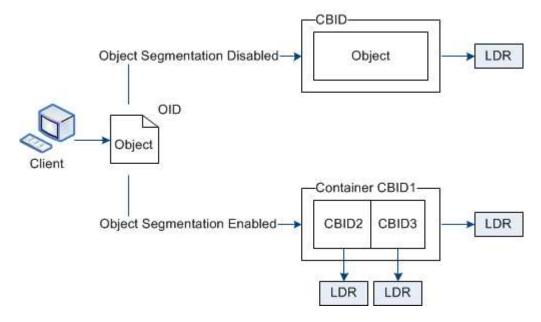
On retrieval of a segment container, the LDR service assembles the original object from its segments and returns the object to the client.
