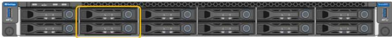
The two solid-state drives (SSDs), indicated by the orange outline, are used for storing the StorageGRID operating system and are mirrored using RAID 1 for redundancy. When the SG100 or SG1000 services appliance is configured as an Admin Node, these drives might be used to store audit logs, metrics, and database tables.
