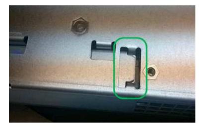
• Incorrect — The battery's metal flange is not inserted into the slot on the controller:
