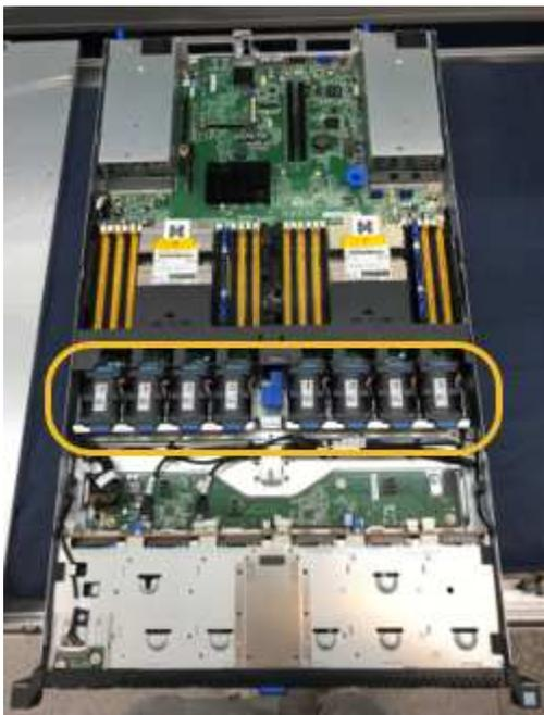
6. Lift the failed fan out of the chassis.
