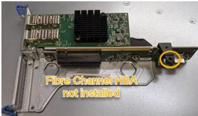
5. Position the riser assembly in the chassis, making sure that it aligns with the connector and guide pin on the system board; then, insert the riser assembly.
