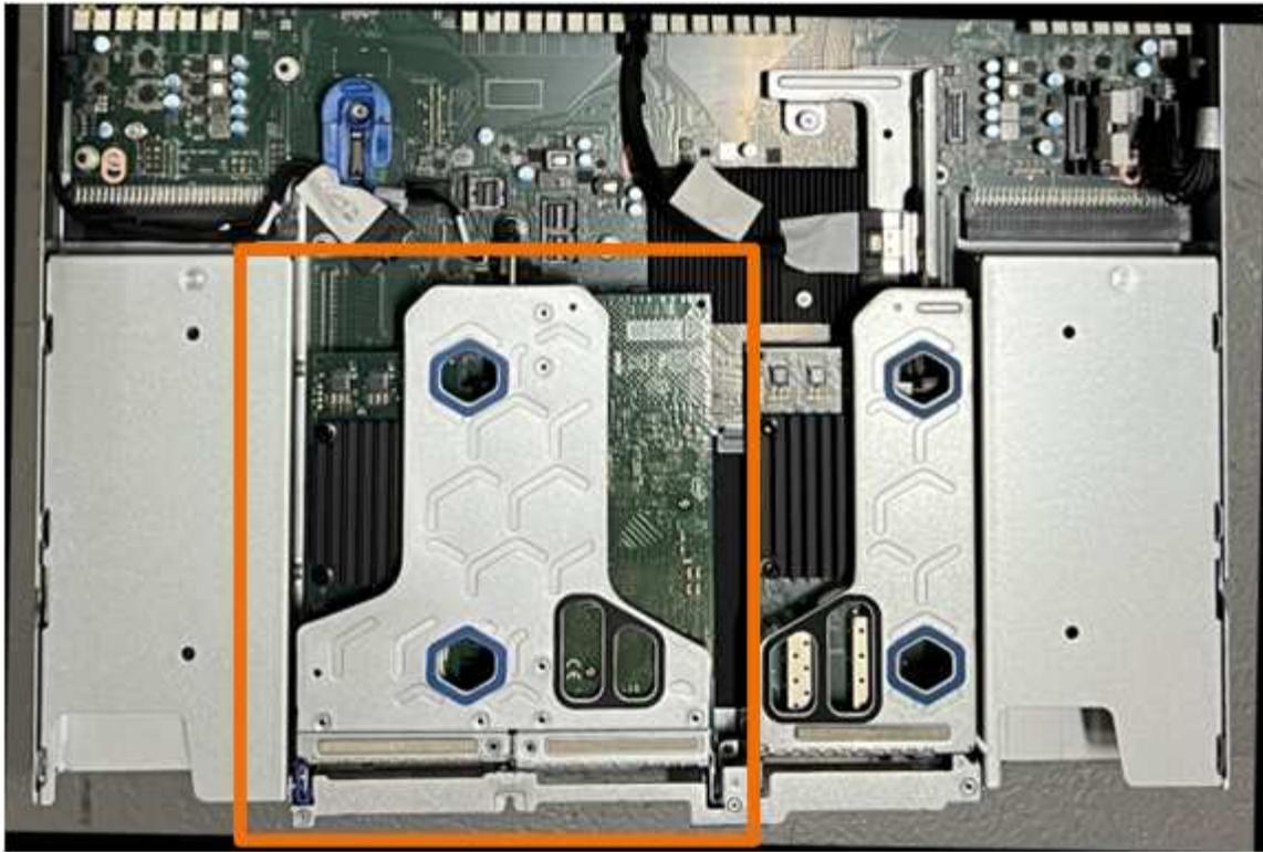
3. Grasp the riser assembly through the blue-marked holes and carefully lift it upwards. Move the riser assembly toward the front of the chassis as you lift it to allow the external connectors in its installed NICs to clear the chassis.
