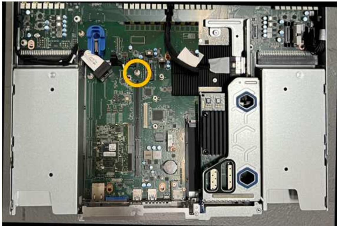
6. Position the riser assembly in the chassis, making sure that it aligns with the connector on the system board and guide pin.
