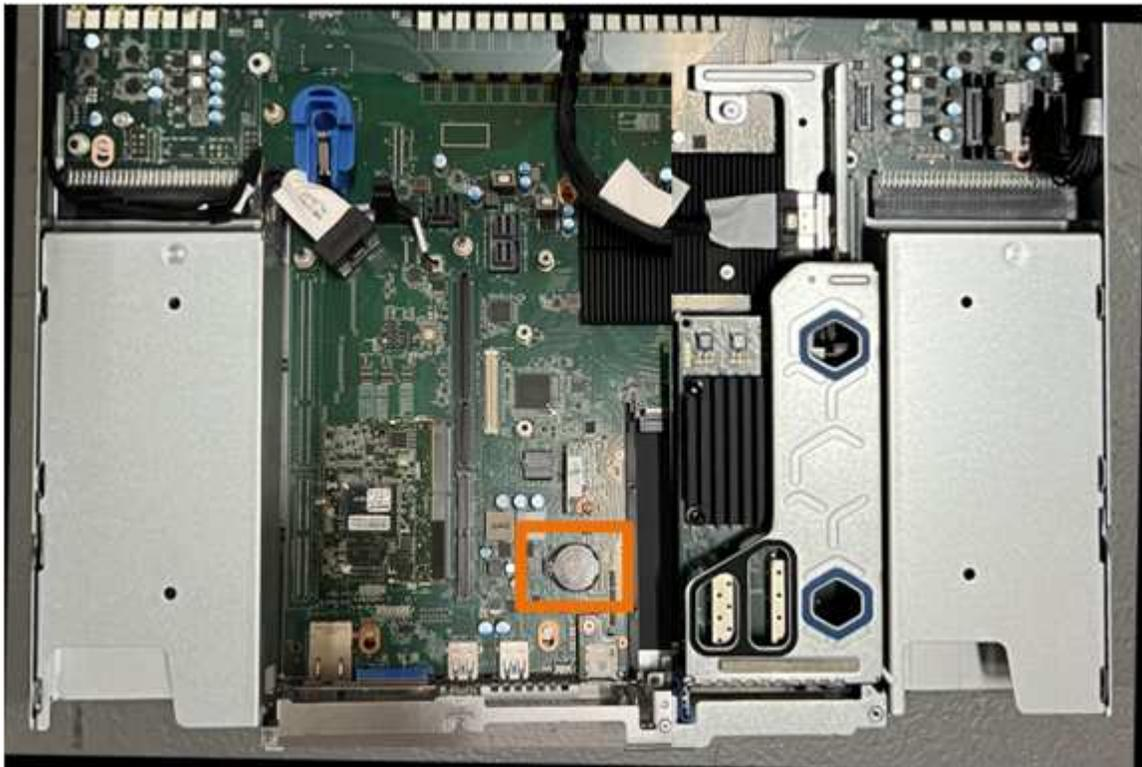
6. Use your finger or a plastic pry tool to press the retaining clip (highlighted) away from the battery to spring it from the socket.
