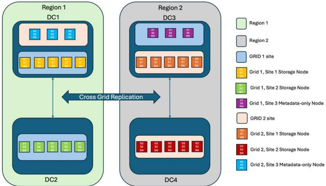
This solution with four separate locations provides complete redundancy of two separate StorageGRID systems maintaining an RPO of 0 and will make use of both multi-site synchronous replication, and multi-grid asynchronous replication. Any single site can fail while maintaining uninterrupted client operations on both StorageGRID systems.
