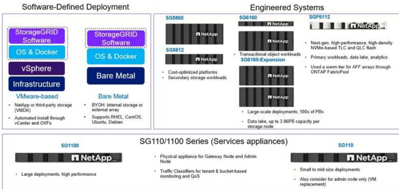
StorageGRID consists of a collection of nodes placed into a site topology. A site in StorageGRID can be a unique physical location or reside in a shared physical location as other sites in the grid as a logical construct. A StorageGRID site should not span multiple physical locations. A site represents a shared local area network (LAN) infrastructure and failure domain.
