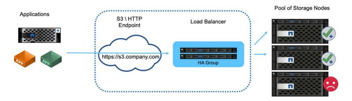
The figure shows the StorageGRID provided load balancer, but the concept is the same for third-party load balancers. Applications establish an HTTP session using the VIP on the load balancer and the traffic passes through the load balancer to the storage nodes. By default, all traffic, from application to load balancer, and from load balancer to storage node is encrypted through HTTPS. HTTP is a supported option.
