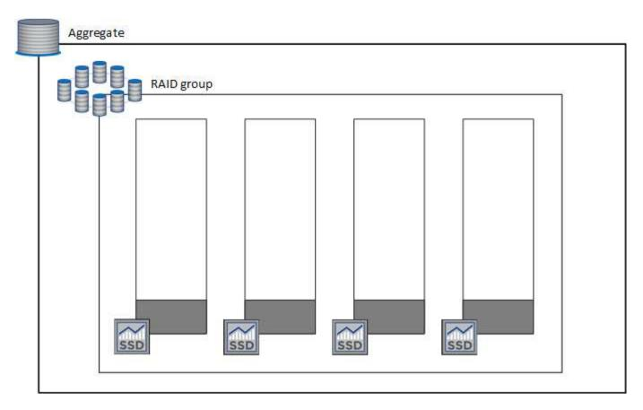
When BlueXP creates an aggregate, it starts with one RAID group. If additional capacity is needed, BlueXP grows the aggregate by increasing the capacity of all disks in the RAID group by the same amount. The capacity increase is either a minimum of 256 GiB or 10% of the aggregate's size.
