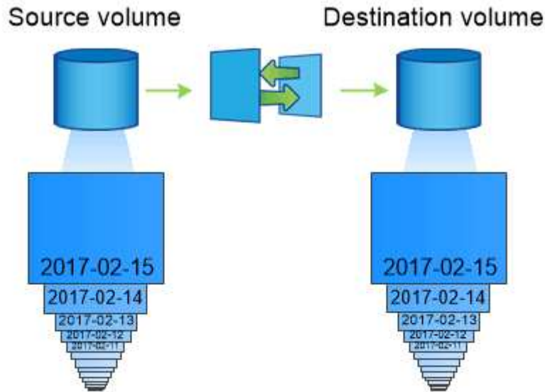
A SnapMirror data protection relationship mirrors the Snapshot copies available on the source volume.
