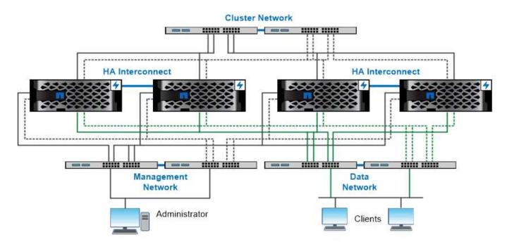
The network architecture for an ONTAP datacenter implementation typically consists of a cluster interconnect, a management network for cluster administration, and a data network.
