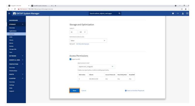
4.5 This will now create the FlexCache volume on the Cloud Volumes ONTAP instance on Google Cloud as a cache volume for the on-premises source data volume. You can view the details by clicking on the name of the FlexCache volume as shown below.
