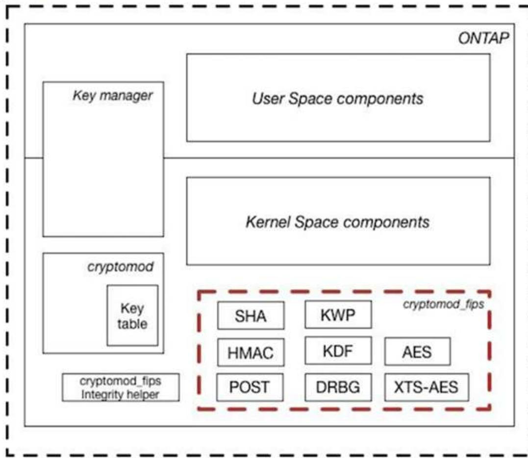
Figure 1 - Block Diagram
