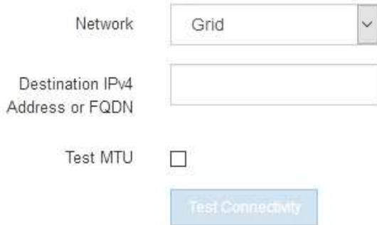
The screenshot shows a web interface for configuring a ping and MTU test. It includes three main input areas: a dropdown menu for 'Network' with 'Grid' selected, a text input field for 'Destination IPv4 Address or FQDN', and a checkbox for 'Test MTU' which is currently unchecked. Below these fields is a blue button labeled 'Test Connectivity'.
